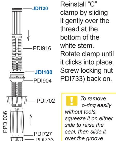
**!** To remove o-ring easily without tools, squeeze it on either side to raise the seal, then slide it over the groove.
