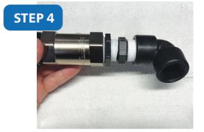
Thread the **3/4**" female to female elbow to the nipple.
