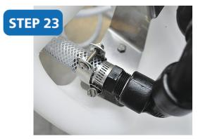
To install the **hose** onto the **hose barb**, place the **hose clamp** over **hose**. Spread support clamp on cart and attach hose with clamp onto the **hose barb**. Tighten clamp with flat head screw driver. Using a Phillips head screwdriver, tighten support clamp using hardware provided with cart.
