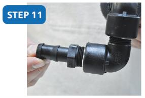
Take the **3/4**" **hose barb** and attach to the thread on the **elbow**.
