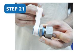
Wrap **thread seal tape** around the threads of the **stainless steel hose adapter** supplied with the cart.
