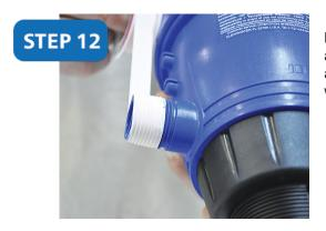
Before installing the assemblies, thread the inlet and outlet of the Dosatron with **thread seal tape**.
