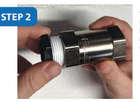
To assemble the inlet side, insert a **1**" to **3/4**" reducer bushing to each side of the stainless steel flow restrictor.
