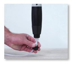
**Step 26:** Insert the hose into the barb and hand tighten the nut. Pull on the hose to make sure it's connected securely.
