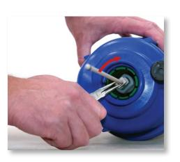
**Step 22:** To install the new plunger assembly (Part #: 8PJ074), use the needle nose pliers to align the top of the plunger with the retainer. Then twist it a quarter turn clockwise to lock.
