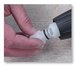
**Step 18:** You can now install the new check valve assembly (Part #: PJDI140) into the stem and reinstall the check valve nut.
