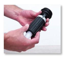
Step 8: Unscrew and remove the adjusting nut.
