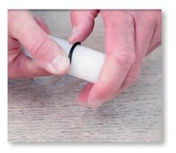
**Step 13:** Then, remove the injection stem o-ring (Part #: JDI120) by pinching and rolling it off the white stem. Install the new o-ring into the groove.
