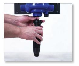
**Step 23:** Carefully slide the injection stem assembly onto the plunger.
