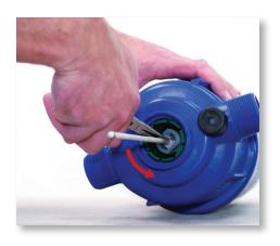
**Step 21:** Position the needle nose pliers near the top of the plunger and carefully twist it a quarter turn counterclockwise and disconnect. Discard the old plunger.
