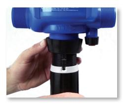
Step 2: Unscrew the injection stem nut and remove.
