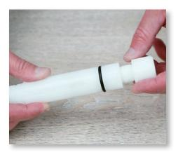
**Step 11:** Next, pick up the white injection stem and unscrew the upper insert and remove.
