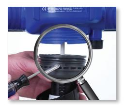
**Step 24:** Align the notches in the lower part of the blue body with the teeth on the top of the injection stem assembly. Slide the two parts together, then hand tighten the injection stem nut. Set the unit aside.
