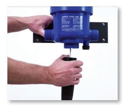
**Step 3:** Pull the injection stem straight out from the body of the injector. Set the unit aside.
