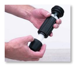
Step 6: Unscrew and remove the lock nut.
