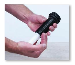
**Step 9:** Push the white injection stem up and out of the black sleeve. Use a towel and dry the outer portion of white injection stem and the top of the black sleeve.
