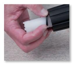
**Step 16:** Replace the "C" clamp by sliding it over the threads at the bottom of the white stem. Rotate the clamp until it clicks into place.
