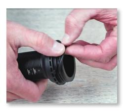
**Step 10:** Remove the injection sleeve o-ring (Part #: JDI100) by pinching and rolling it off the black sleeve. Install the new o-ring into the groove. Set the black sleeve aside.
