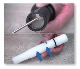
**Step 14:** To reassemble, align the groove in the white injection stem with the tooth inside the lower portion of the black sleeve and slide the stem down as far as possible.
