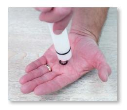
**Step 12:** Flip the white injection stem upside down so the upper insert o-ring falls out into your hand. Discard the upper insert o-ring and replace with a new one (Part #: 20J006). Reinstall the top.
