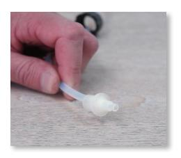
**Step 25:** Before installing the suction hose, slide the ferrule back and cut a half inch off the top of the hose. Reposition the ferrule.
