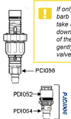
If only the check valve barb (PDI054) comes out, take a pencil (eraser side down) through the top of the injection stem and gently push the check valve guide (PDI052) out.
